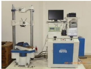
Universal Testing Machine for Tensile 10 Ton
