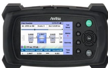
Optical time-domain Reflectometer (MT9090A from Anritsu)
