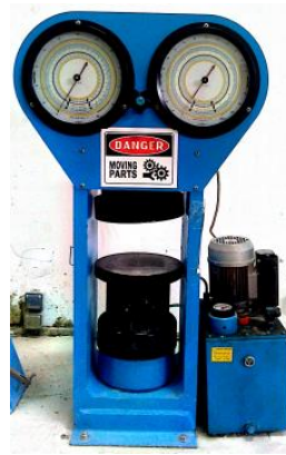
Machine for Measurement of Compressive strength of R.C. Cubes
