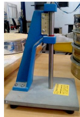
Machine for measurement of Cement Hardening
